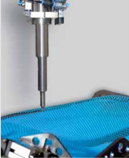
← Robotically guided oscillator system with cutting horn
